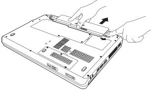
(Sample Illustration) Removing the battery
